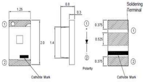
All dimensions in millimetres with +/- 0.1mm tolerance unless otherwise stated.
